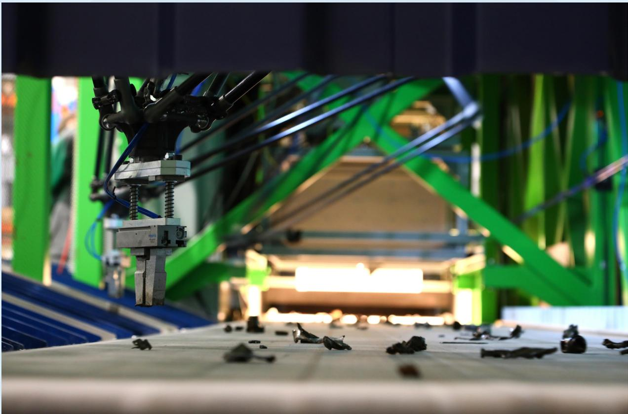
Industrial progress independent of LIFE PlasPLUS, resulted in the emergence of an XRF technology to separate FRP from WEEE and ELV waste plastic streams. To align itself on these new developments, the LPP partners relied on the REDWAVE XRF sorting technology. Two XRF sorting campaigns were successfully conducted in February 2021 and April 2022 to produce 1.2 tons of high-grade bearing Sb plastic.
