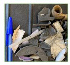
The so called "Drainaplus" fraction of Comet Treatments containing plastics with brominated flame retardants and Antimony (FR) is being characterized with an X Ray gun to isolate FR-bearing fragments. These fragments will be sent to the University of Liège as control samples for the PICKIT pilot.
